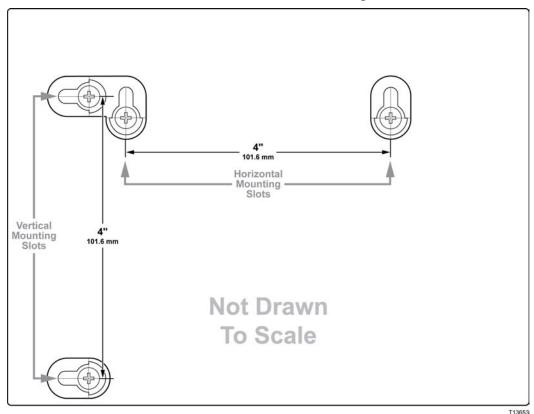
The following illustration shows the location and dimensions of the wall-mounting slots on the bottom of the modem. Use the information on this page as a guide for mounting your modem to the wall.
